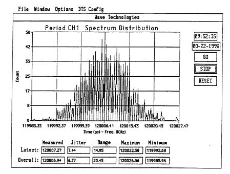
Spectrum Analysis-HP8110A PRBS=7 (50 Mhz Output, Filtering around 120ns period, With Accumulation)
