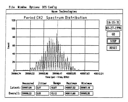
Spectrum Analysis--Q/2 Period Jitter (50 Mhz In, Vcc=5.00v, Supplier A)
