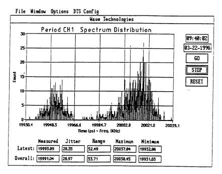
Spectrum Analysis--HP8110A PRBS=7 (50 Mhz Output, Filtering around 20ns period)
