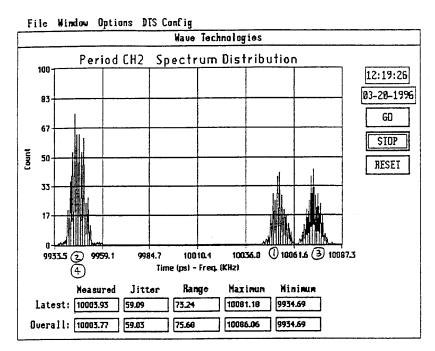
Spectrum Analysis-2XQ Period Jitter (50 Mhz in, Vcc=5.00v, Supplier B NEW)
