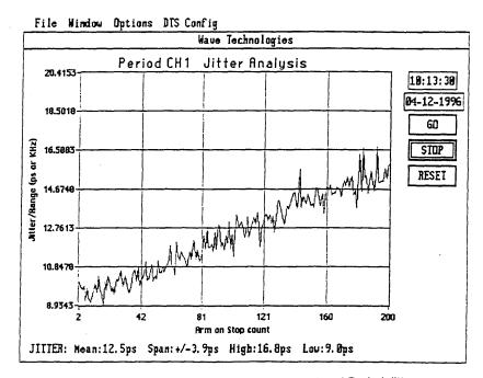
Jitter Analysis-Input Reference Accumulated Period Jitter (19.5 Mhz In, Vcc=5.25v, Supplier B OLD)
