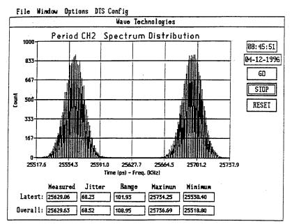
Spectrum Analysis--2XQ Period Jitter (19.5 Mhz In, Vcc=5.25v, Supplier B OLD)
