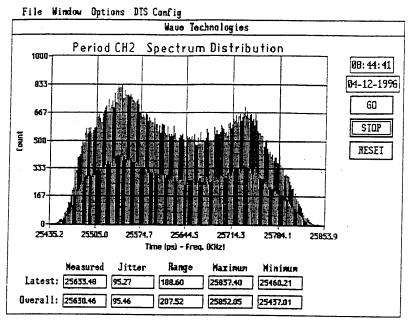
Spectrum Analysis--2XQ Period Jitter (19.5 Mhz In, Vcc=5.00v, Supplier B OLD)
