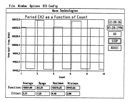
Function Analysis-2XQ Period vs. Counts (50 Mhz In, Vcc=5.00v, Supplier B NEW)
