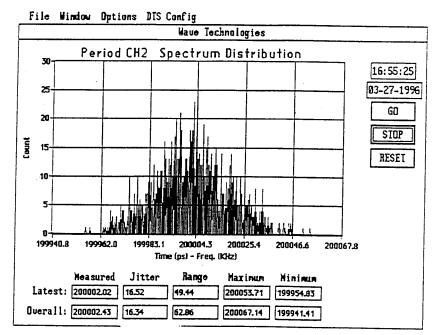
Spectrum Analysis--Q/2 Period Jitter (10 Mhz In, Vcc=5.00v, Supplier A)
