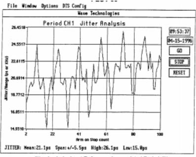
Jitter Analysis-Input Reference Accumulated Period Jitter (23 Mhz In, Vcc=5.00v, Supplier B NEW)
