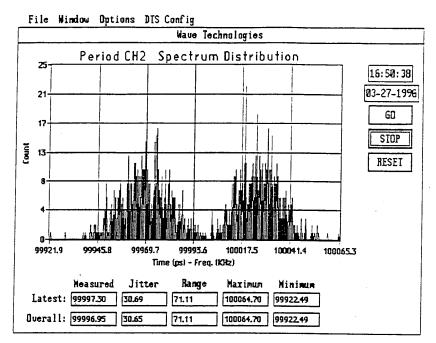
Spectrum Analysis--Q4 Period Jitter (10 Mhz In, Vcc=5.00v, Supplier A)
