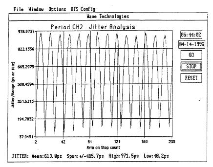
Jitter Analysis-Q4 Accumulated Period Jitter (19.5 Mhz In, Vcc=4.75v, Supplier B OLD)
