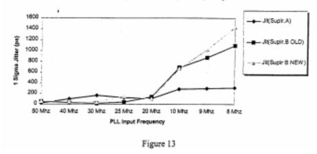
The above PLL output jitter behavior suggests that a finer frequency sweep (especially at lower input frequency) on the PLL input may be revealing. When this was performed on the Supplier B OLD design, a significant output jitter sensitivity was noticed when the input frequency was set to 19.5MHz. Not only was there an input frequency sensitivity, but the Vcc level also had a significant influence on output jitter behavior.
