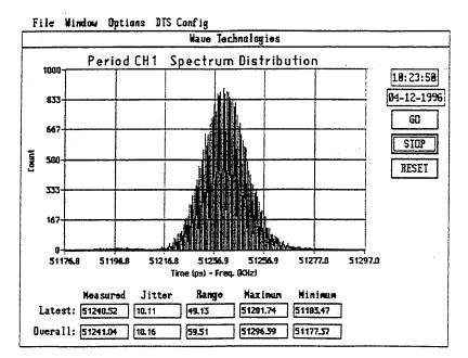
Spectrum Analysis-Input Reference Period Jitter (19.5 Mhz In, Vcc=4.50v, Supplier B OLD)
